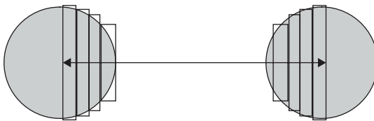
Figure 2 Schematic showing how interactions between surfaces can be used to estimate interactions between particles of specific shapes.
